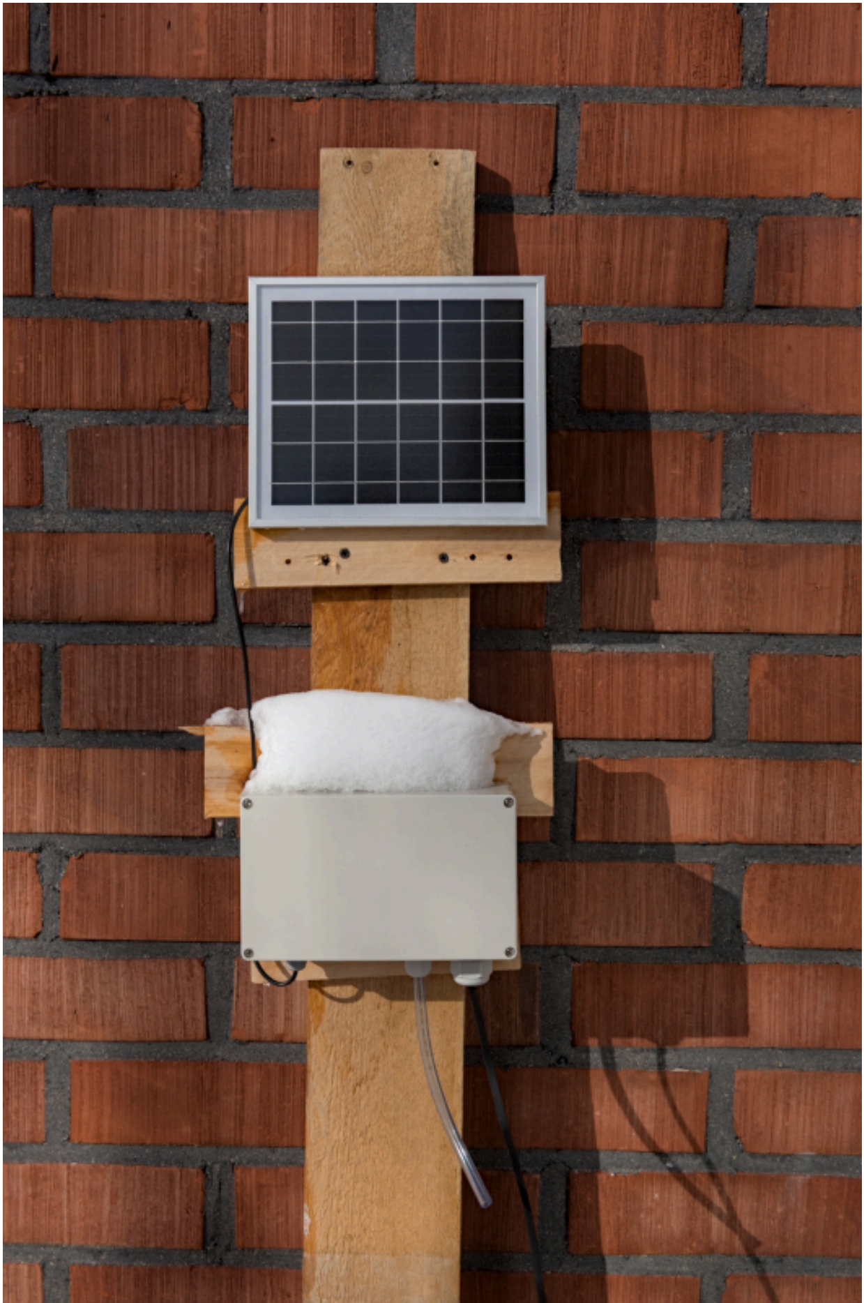
Fig 1: Citizen science air quality measuring station powered with a solar panel © Gerald Žojer, 2024.
